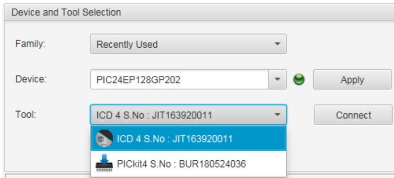
5. Click the **Connect** button (next to the Tool name) to establish a connection between the IPE and the tool.
